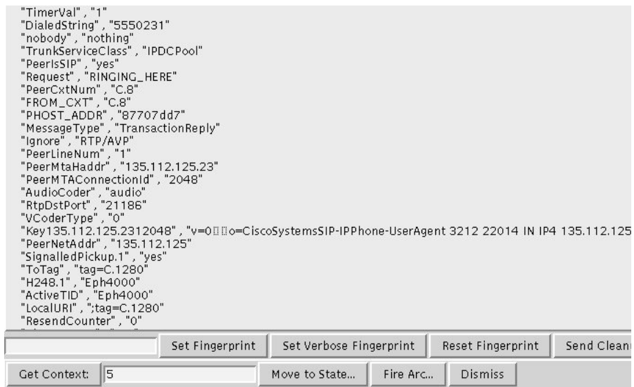
Figure 8.2: Name/Value Pairs from an H.248 VoIP Session
